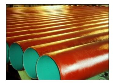
The ceramic modified epoxy lining offers exceptional abrasion resistance and a low permeation rate for an impenetrable barrier to H2S and other sewer gases. And its high-build application ensures fast and efficient throughput of pipe and fittings during the manufacturing process.
