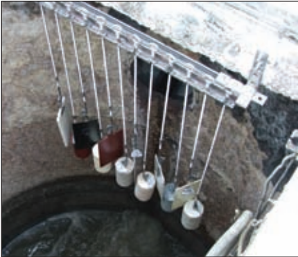
Fig. 4: Typical testing site with carbon steel and concrete samples suspended in severe wastewater headspace environment.
