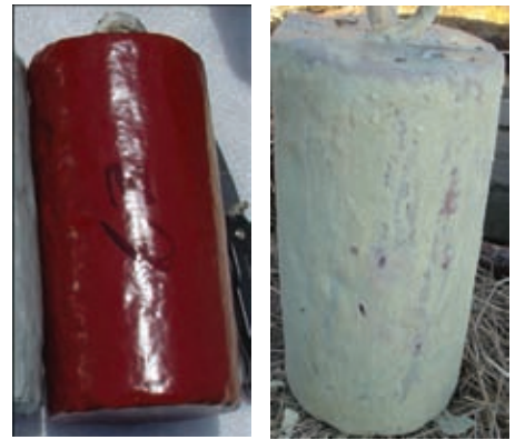
Fig. 13: South TX: 55% volume solids polyamide epoxy applied at 17 mils DFT to concrete cylinder panel before 12-month exposure (left) and following 12-month exposure (right).
