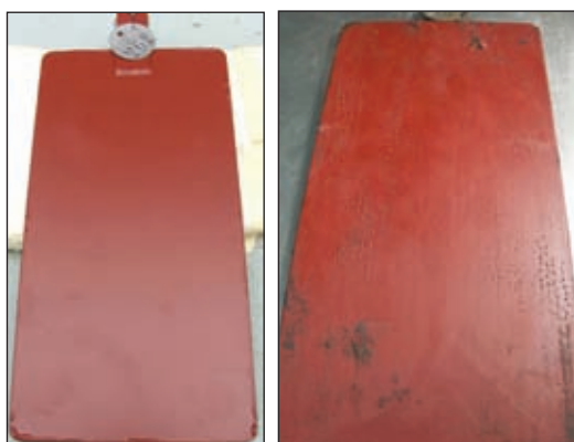
Fig. 9: Midwestern US: Polyamide epoxy applied to carbon steel panel at 11 mils DFT before 12-month exposure (left) and following 12-month exposure, cleaned (right). Note moderate blistering following exposure.
