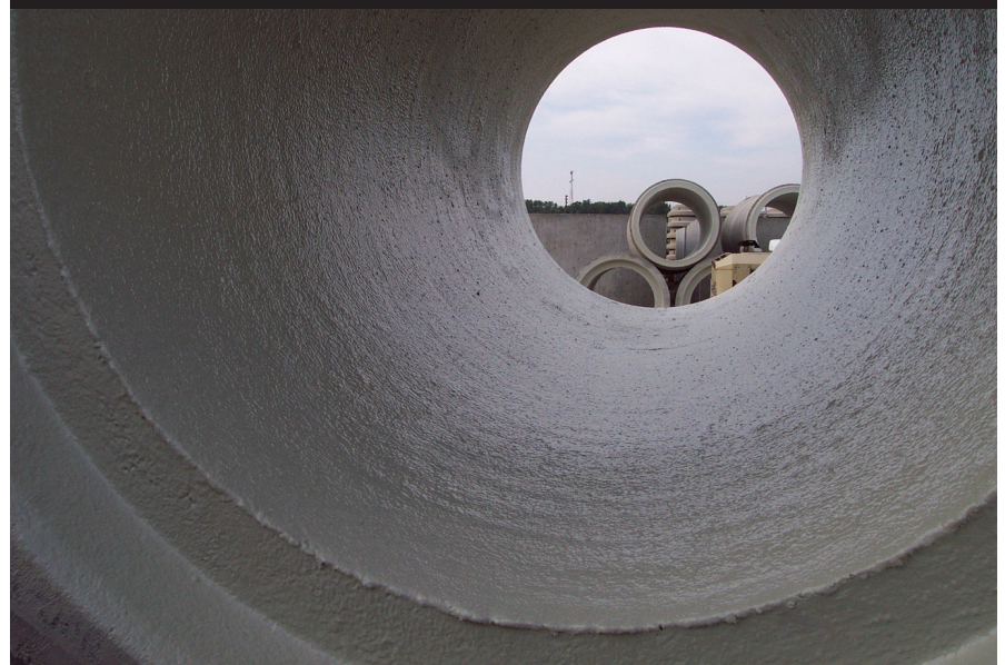
Typical 48-in. precast sewer interceptor lined with a 100% solids, fiber-reinforced polyamine epoxy for elevated H_2S resistance.
