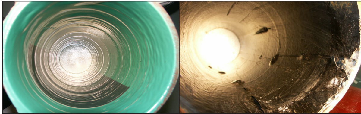
Figure 4: Comparison of Series 431 and ceramic novolac epoxy after 30 day pipe acid immersion test
