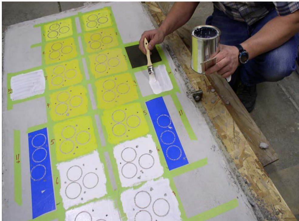
Test Slab; untreated concrete left side, Ashford Formula treated concrete right side.
