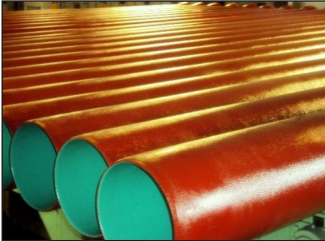
The ceramic modified epoxy lining offers exceptional abrasion resistance and a low permeation rate for an impenetrable barrier to H<sub>2</sub>S and other sewer gases. And its high-build application ensures fast and efficient throughput of pipe and fittings during the manufacturing process.
